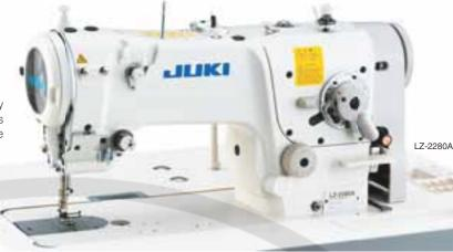
Two kinds of gauges can be selected in accordance with the application of the machine: an A-type gauge with a zigzag width of 5 mm, and a B-type gauge with a zigzag width of 8 mm.
